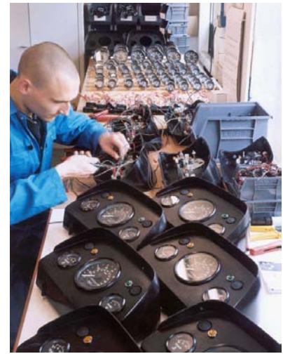
Manufacture of Bedford instrument binnacles.
